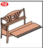
20. Cut the bottom from your 1/4" plywood or hardboard to shape or to fit the rabbets in the bottom. Notch the corners as required to fit around the legs, and install using glue and small screws or finishing nails. Now simply go over the completed bench looking to fill screw holes or to give it a final sanding to perfection. Then you can stain, varnish or paint your Deacon's Bench as you wish.
