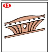
14. Place the top rail over the tenons of the back slats. You might have to support the outer slats with tape or clamps to keep them in proper position. Attach the top rail with glue and plugged screws. In the slot, fill the gaps between the slats with blocks cut to fit, as was done with the bottom rail. Again, glue the blocks, but not the slats themselves.
