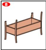
From the solid oak stock, cut back slats to a design created or create one of your own. Whichever pattern you use, use a jig saw or band saw to cut out the appropriate profiles.
