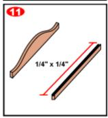
12. Rip strips of scrap oak 1/4" wide x 1/4" thick. Working on a flat tabletop, arrange the back parts into position by inserting the slats into the slots in the rails. Fill in the gaps between them with blocks cut from these strips. Glue the blocks, but the slats should be loose. The gaps between the parts should be 3/4". When the glue is dry, remove the slats and sand the edges of the rails, with the filler blocks, smooth. Round the edges slightly by sanding.
