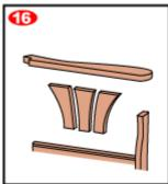
17. Drill 1/4" holes in the top and bottom edges of the side slats in order to assemble using 1/4" fluted dowels. Use dowel centers to transfer the dowel positions to mating parts. Apply glue to the bottom dowels and glue the side slats into position on the sides.
